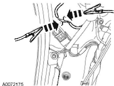
Fig. 218: Attaching Wire Of Jumper Harness To Wire Of Safety Canopy/Side Air Curtain Module
